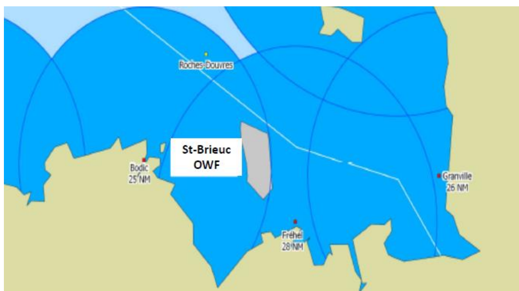
Figure 15: Saint-Brieuc (France) OWF project and the different VHF coverages (GMDSS sea area A1 in blue) around VHF CRS
